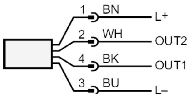
OUT1: Switching output / IO-Link
