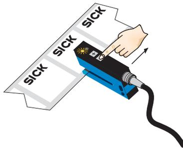
Press both the “+” and “-” buttons together, hold > 1 s and then release the teach-in buttons. The red LED flashes.
